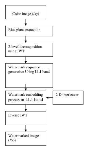
Fig.3: Block diagram for watermark Embedder
